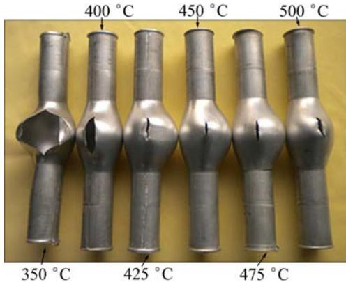
Fig. 3 Workpieces obtained at different temperatures
