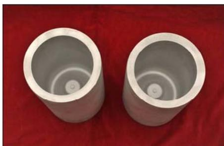
**Fig. 7** Thixoformed barrel-shaped components with thin walls by RAP route (four-pass CCDF and partial remelting)
