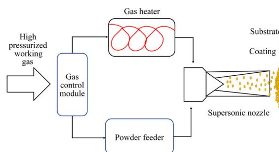
**Fig. 6** Schematic diagram of cold spray process
