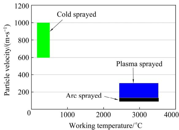
**Fig. 8** Working temperature and particle velocity of various spray techniques [113]
