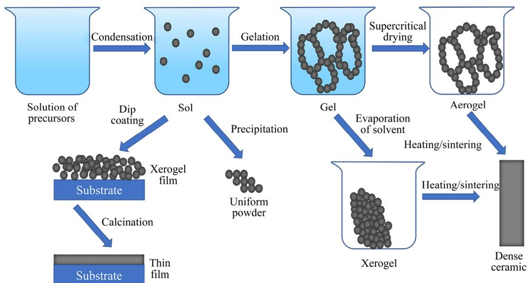
**Fig. 5** Schematic illustration of sol–gel process and different products of different stages
