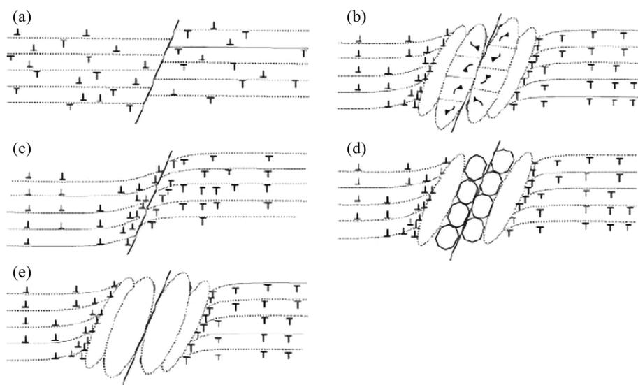
**Fig. 9** Schematic diagram showing proposed mechanism of dynamic recrystallization in deposited particles during cold spraying [121]: (a) Substrate with low dislocation density before spraying; (b) Dislocation density with spraying processing; (c) Formation of elongated subgrains observed due to accommodated dislocations; (d) Dynamic recrystallization (Elongated subgrains were divided into equiaxed subgrains); (e) Formation of ultrafine grains
