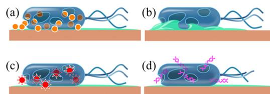
**Fig. 3** Four stages of contact killing [20] (Stages (a–d) represent copper dissolution and ions release, bacterial copper homeostasis and cell membrane failure, cell damage caused by copper ions and ROS, and DNA degradation, respectively)
