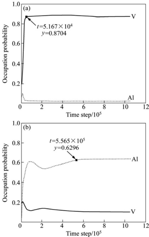
Fig. 6 Variations of average occupation probability values of Al and V in different diffusion channels: (a) DO<sub>22</sub> channel; (b) L<sub>12</sub> channel
