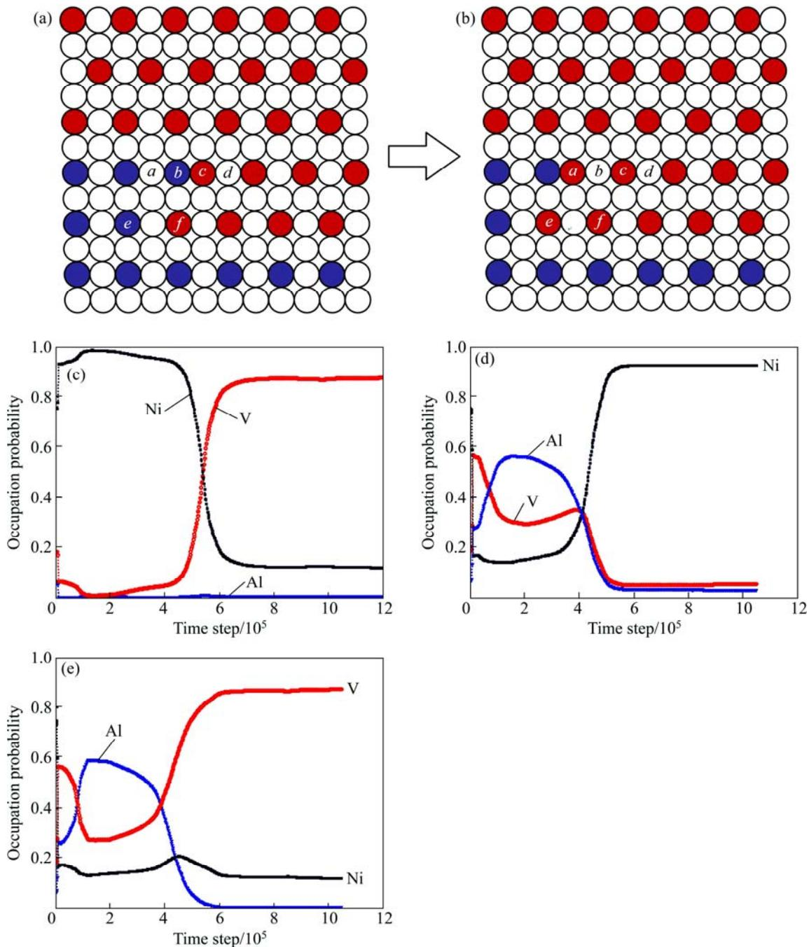
**Fig. 4** Evolution of interface between  $L1_2$  and  $DO_{22}$  (a,b) and occupation probabilities of atoms at interface in positions  $a$  (c),  $b$  (d) and  $e$  (e)
