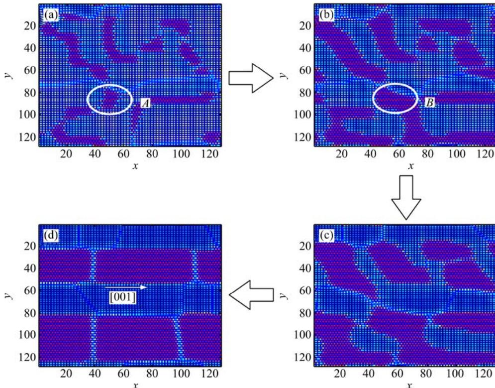
**Fig. 2** Evolution of morphology for  $Ni_{75}Al_{6.7}V_{18.3}$  alloy at 1100 K at different time steps (Horizontal and ordinate coordinate are lattice positions in  $[001]$  and  $[100]$ , respectively): (a)  $t=4\times 10^4$ ; (b)  $t=8\times 10^4$ ; (c)  $t=3\times 10^5$ ; (d)  $t=10.5\times 10^5$
