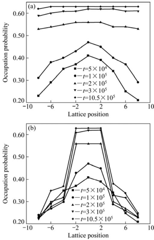
Fig. 5 Occupation probability of Al for L<sub>12</sub> channel in two directions: (a) [001]; (b) [100]
