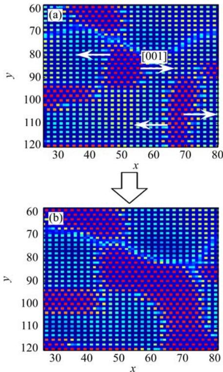
**Fig. 3** Evolution of oriented growth for DO<sub>22</sub> from  $t$  of  $4 \times 10^4$  (a) to  $8 \times 10^4$  (b)
