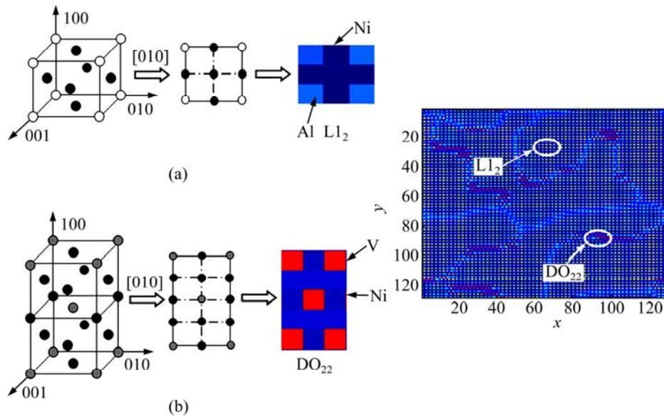
**Fig. 1** Morphology of  $Ni_{75}Al_{6.7}V_{18.3}$  alloy at 1100 K when  $t=2.2\times 10^4$  and corresponding relation between simulation results and lattice structures projected in direction  $[010]$  (Horizontal and ordinate coordinates are lattice positions in  $[001]$  and  $[100]$ , respectively): (a)  $Ni_3Al-L_{12}$ ; (b)  $Ni_3V-DO_{22}$
