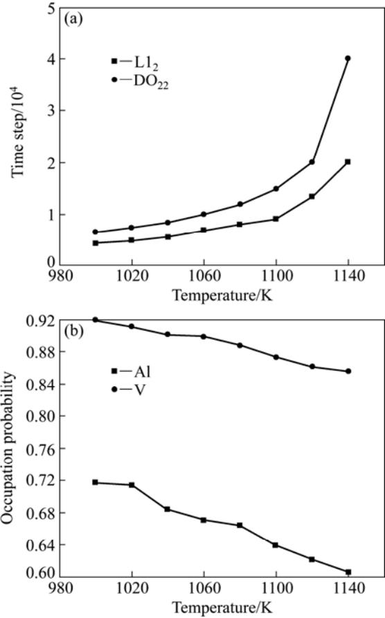
Fig. 7 Evolution of appearing time for two phases (a) and occupation probability of Al and V of Ni<sub>75</sub>Al<sub>6.7</sub>V<sub>18.3</sub> alloy (b)
