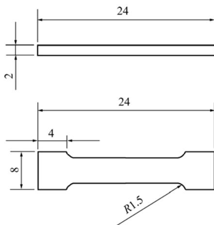
Fig. 1 Schematic diagram of tensile specimens (Unit: mm)
