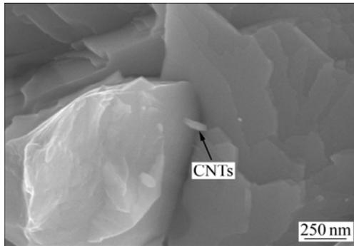
**Fig. 5** CNTs inhibiting cracking of grain boundary of Sn-58Bi-0.03CNTs alloy
