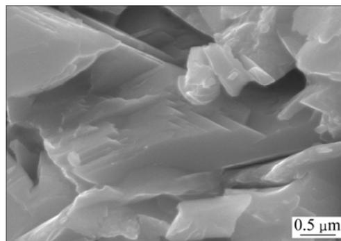
**Fig. 3** Fracture surface of Sn-58Bi alloy
