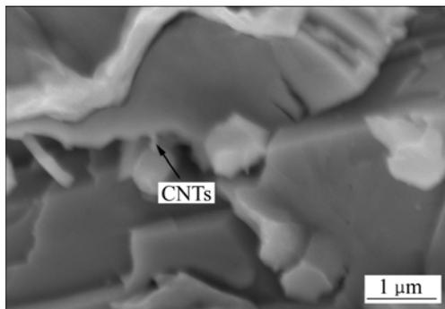
**Fig. 6** Influence of CNTs on fracture mode of Bi rich phase in Sn-58Bi-0.03CNTs alloy
