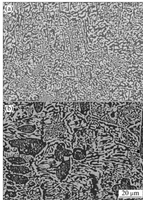
**Fig. 8** Microstructure of Sn-58Bi-0.03CNTs (a) and Sn-58Bi-0.06CNTs (b)
