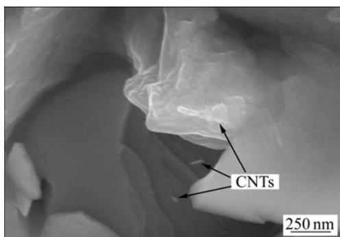
**Fig. 7** Cleavage steps provided by CNTs in Sn-58Bi-0.03CNTs alloy
