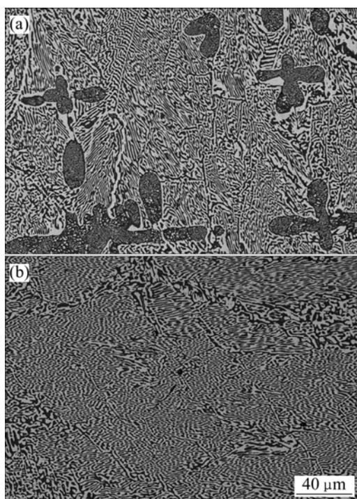
**Fig. 2** Microstructure of composites: (a) Sn-58Bi; (b) Sn-58Bi-0.03CNTs composite
