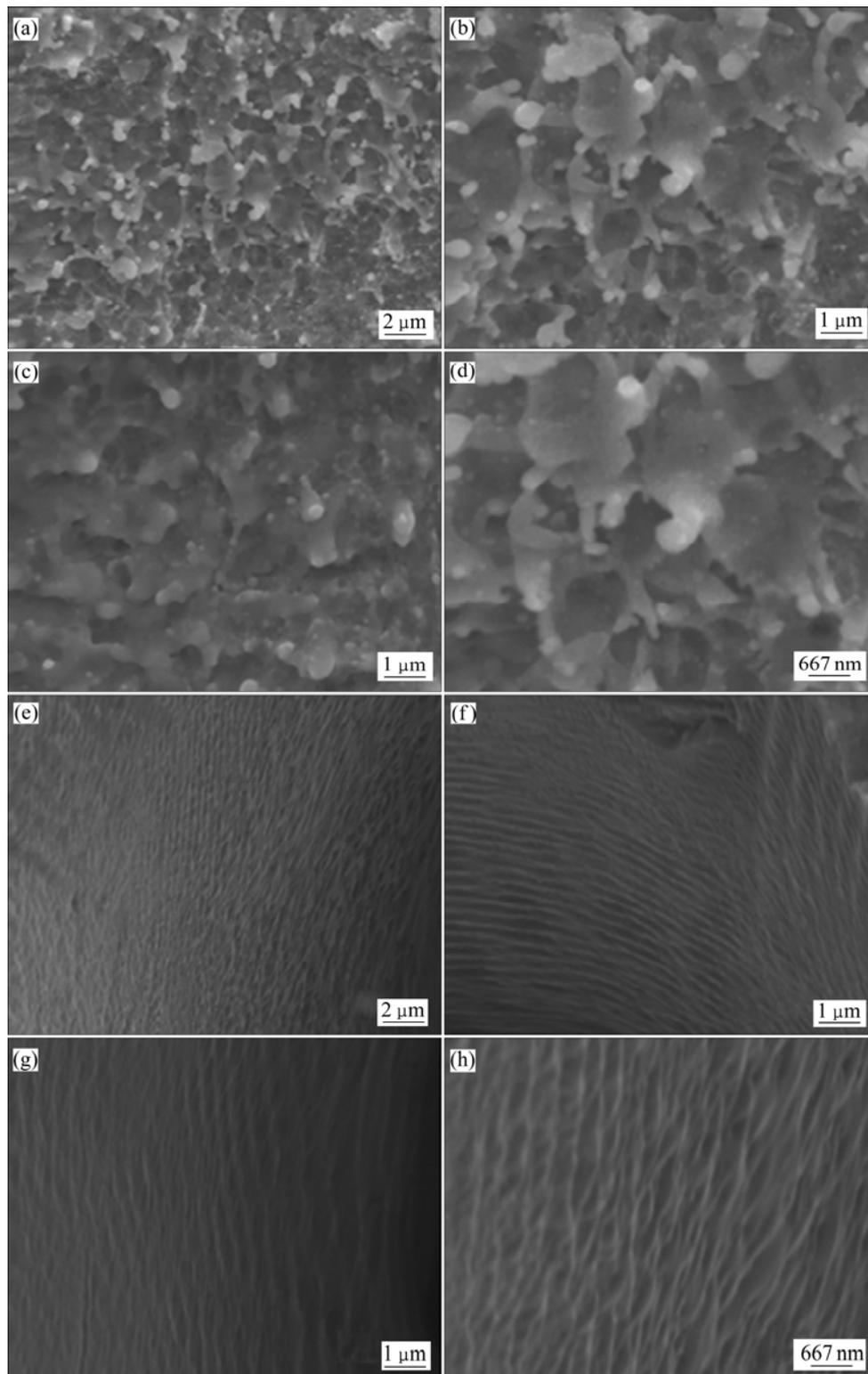
**Fig. 3** SEM images of side-wall surface generated by femtosecond laser drilling of copper substrate (Frequency and displacement of vibration are 500 Hz and 800 nm, and the irradiated energy is 50  $\mu\text{J}/\text{pulse}$ .): (a–d) Without vibration assistance; (e–h) With vibration assistance
