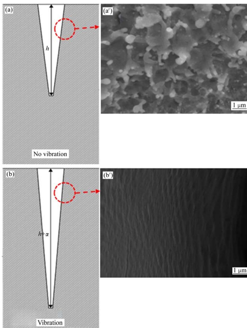
**Fig. 5** Illustration of femtosecond laser-drilled holes and SEM images of deposited materials of wall surface by femtosecond laser machining of copper substrate: (a, a') Without vibration assistance; (b, b') Vibration assistance
