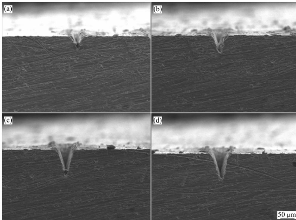
**Fig. 4** Cross-sectional SEM images of copper substrate machined with various displacement vibrations using femtosecond laser with a pulse energy of 50  $\mu\text{J}/\text{pulse}$  and scanning speed of 0.01 mm/s; (a) No vibration; (b)  $D=3.5 \mu\text{m}$ ; (c)  $D=15.7 \mu\text{m}$ ; (d)  $D=16.5 \mu\text{m}$
