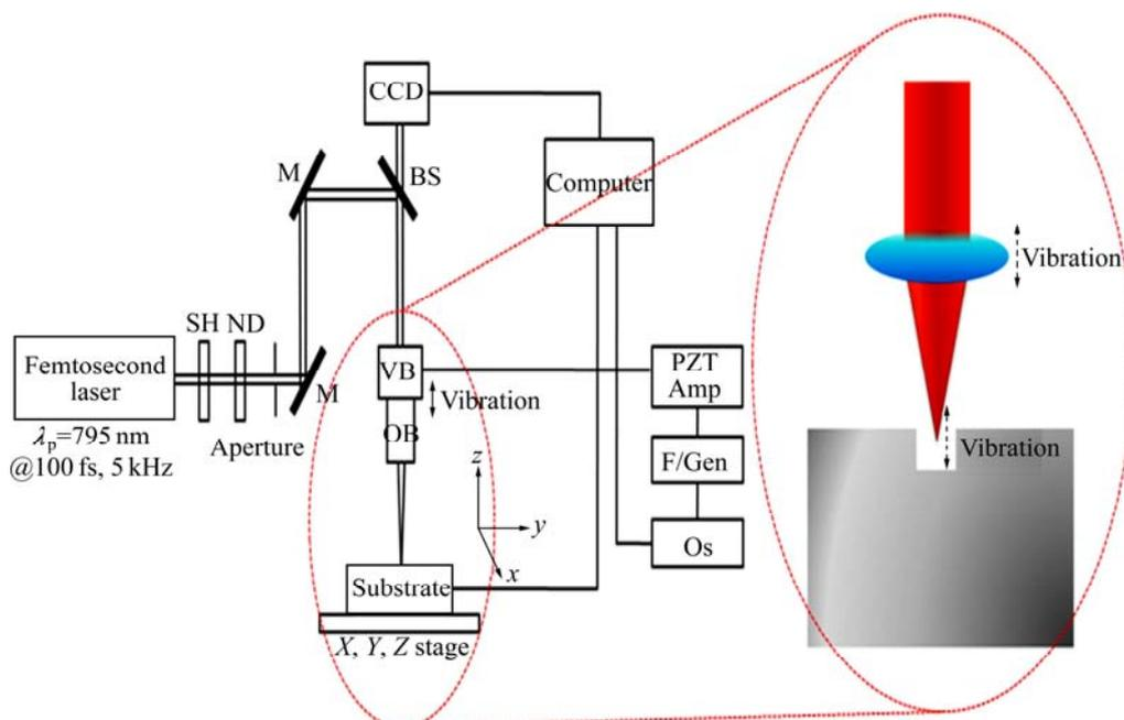
**Fig. 1** Schematic diagram of experimental set-up of vibration-assisted femtosecond laser hybrid machining system (SH—Shutter; ND—Neutral density filter; M—Mirror; CCD—CCD camera; BS—Beam splitter; OB—Objective lens; VB—Vibrator; PZT Amp—PZT Amplifier; F/Gen—Function generator; OS—Oscilloscope)
