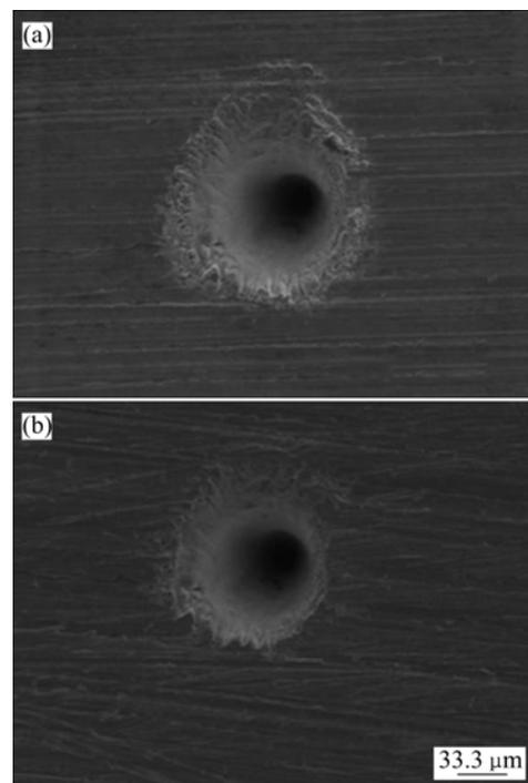
**Fig. 2** SEM images of hole at entrance end drilled without vibration assistance (a) and with vibration assistance (b)
