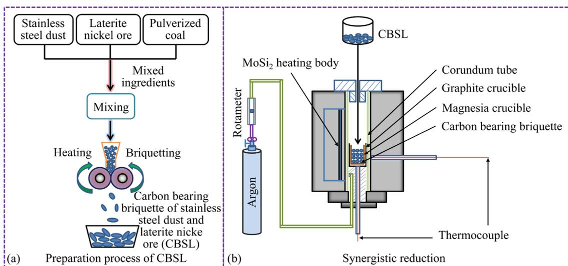
Fig. 2 Process flow charts of CBSL preparation (a) and synergistic reduction natural cooling separation experiment (b)
