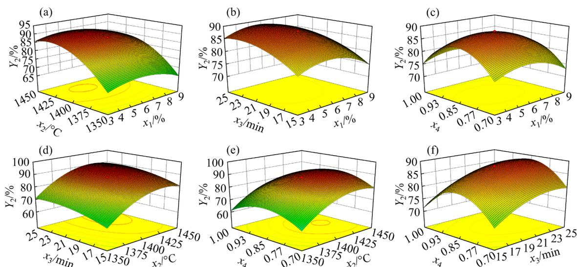
**Fig. 6** 3D response surface of effects of laterite nickel ore addition ( $x_1$ ), reduction temperature ( $x_2$ ), reduction time ( $x_3$ ), and FC/O ( $x_4$ ) on Cr recovery ( $Y_2$ )
