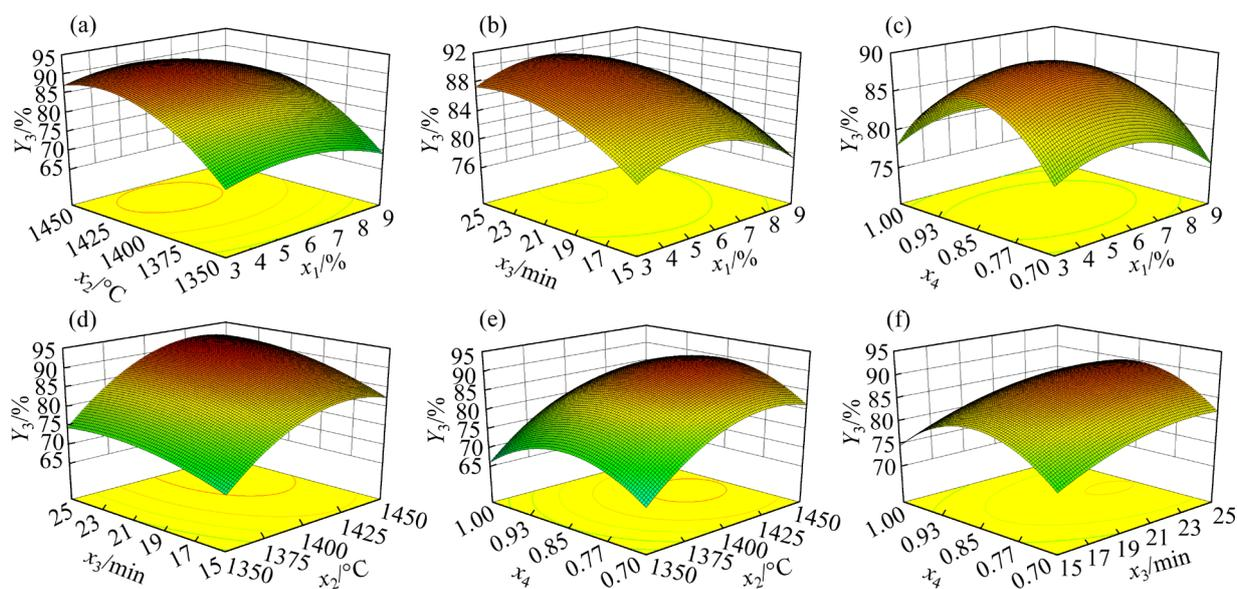
**Fig. 7** 3D response surface of effects of laterite nickel ore addition ( $x_1$ ), reduction temperature ( $x_2$ ), reduction time ( $x_3$ ) and FC/O ( $x_4$ ) on Ni recovery ( $Y_3$ )
