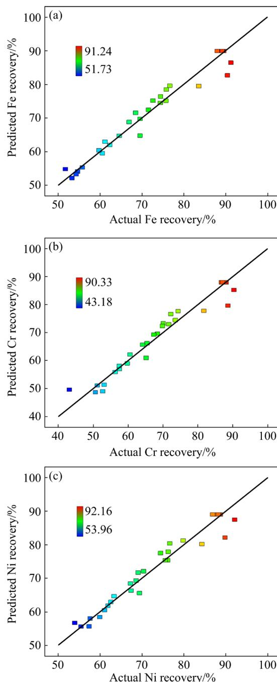
**Fig. 4** Comparison between predicted and actual recovery: (a) Fe recovery; (b) Cr recovery; (c) Ni recovery
