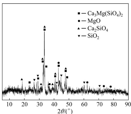
Fig. 9 XRD pattern of reduced slag
