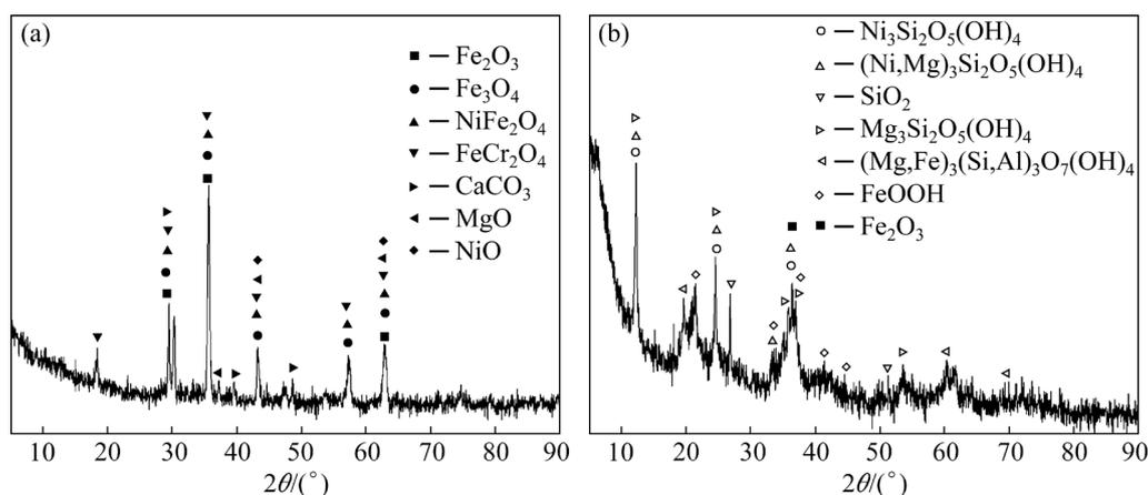
Fig. 1 XRD patterns of stainless steel dust (a) and laterite nickel ore (b)
