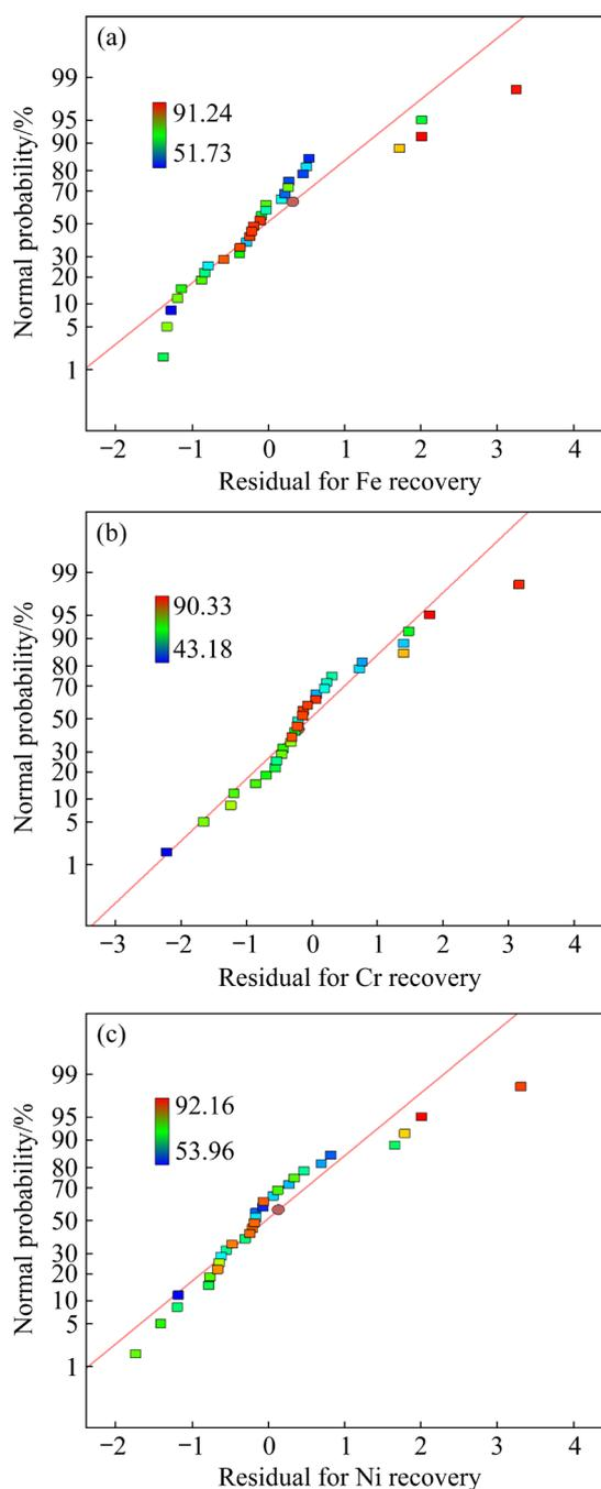
**Fig. 3** Normal probability distribution of residuals: (a) Fe recovery; (b) Cr recovery; (c) Ni recovery
