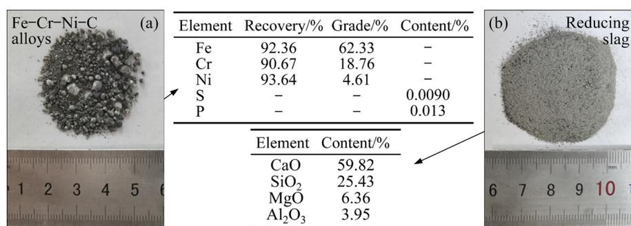
Fig. 8 Analysis of CBSL reduction products under optimized conditions
