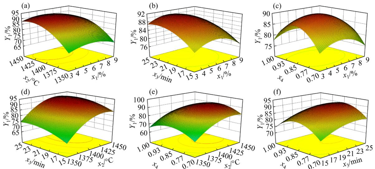
**Fig. 5** 3D response surface of effects of laterite nickel ore addition ( $x_1$ ), reduction temperature ( $x_2$ ), reduction time ( $x_3$ ), and FC/O ( $x_4$ ) on Fe recovery ( $Y_1$ )
