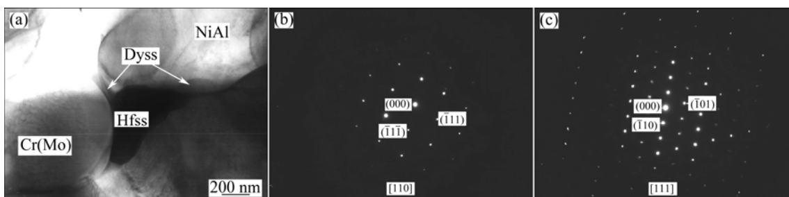
Fig. 5 Bright field TEM image of Hfss and Dyss phases (a); SAED pattern of Hfss phase along [110] zone axis (b); SAED pattern of Dyss phase along [111] zone axis (c)
