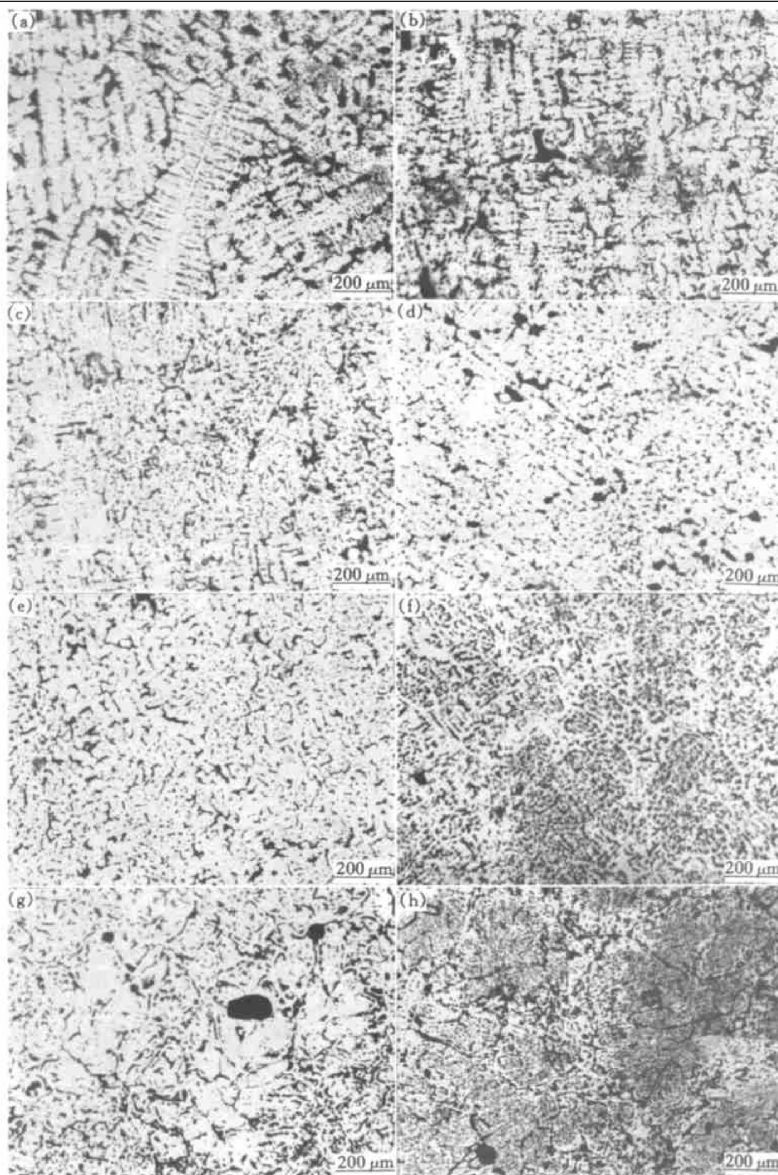
Fig. 2 Solidification microstructures of Ni31.44% Pb monotectic alloy under different undercoolings (a) -\Delta T = 10 K; (b) -\Delta T = 50 K; (c) -\Delta T = 70 K; (d) -\Delta T = 110 K; (e) -\Delta T = 154 K; (f) -\Delta T = 203 K; (g) -\Delta T = 243 K; (h) -\Delta T = 286 K
