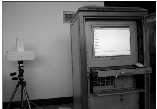
Fig. 2 Vision intelligent console system
