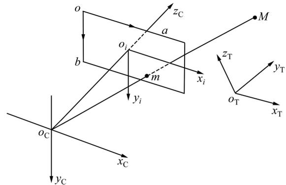
Fig. 1 Image frame, camera frame and object frame
