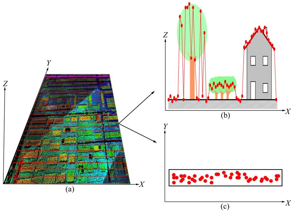
Fig. 2 Divided laser points cloud (a) into Y-coordinate strips (b) and X-coordinate strips (c)
