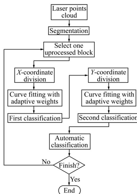
Fig. 1 Flow chart of terrain classification based on adaptive weights for LiDAR data in mining area
