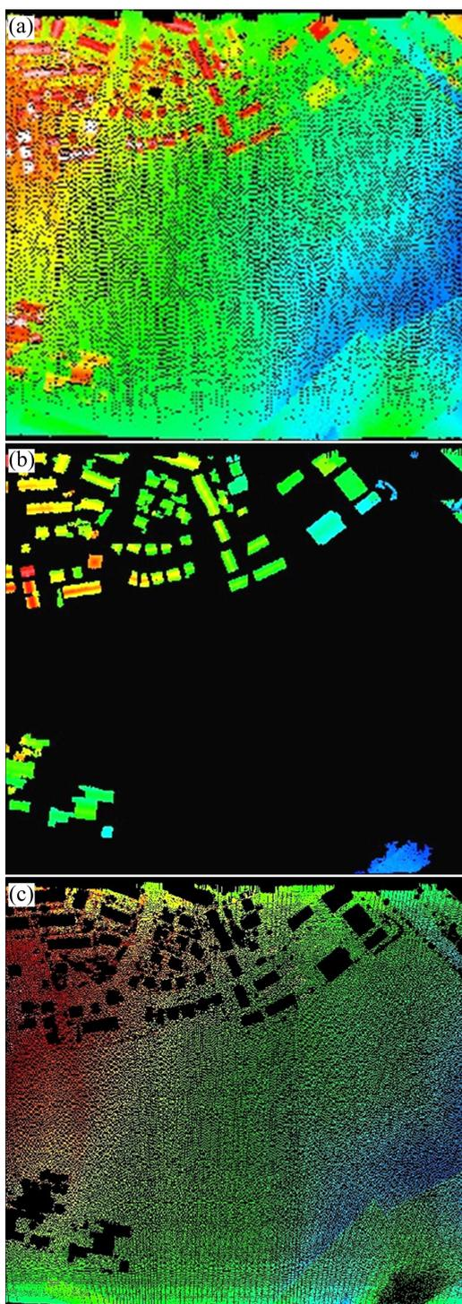
**Fig. 5** Classification result of mining area: (a) Original LiDAR data of mining area; (b) Surface buildings of mining area; (c) Terrain data of mining area
