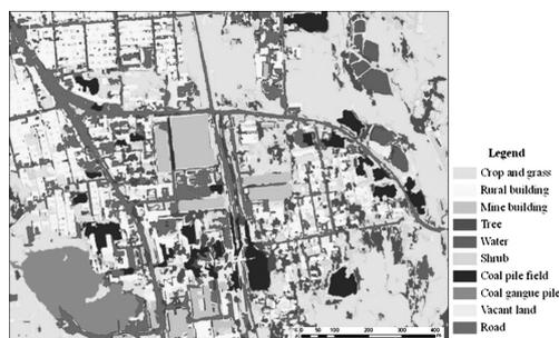
**Fig. 5** Coal mine area lands cover information extraction result
