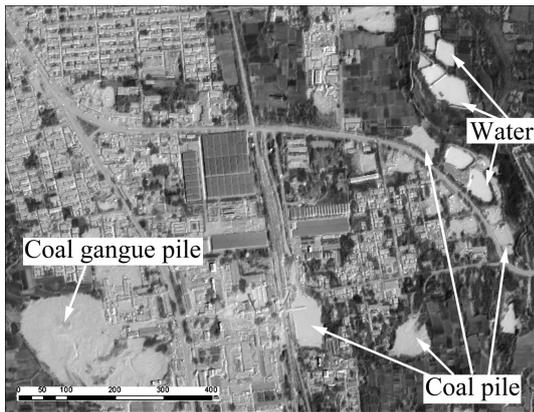
**Fig. 4** Coal pile and water body looking similar in NDWI image
